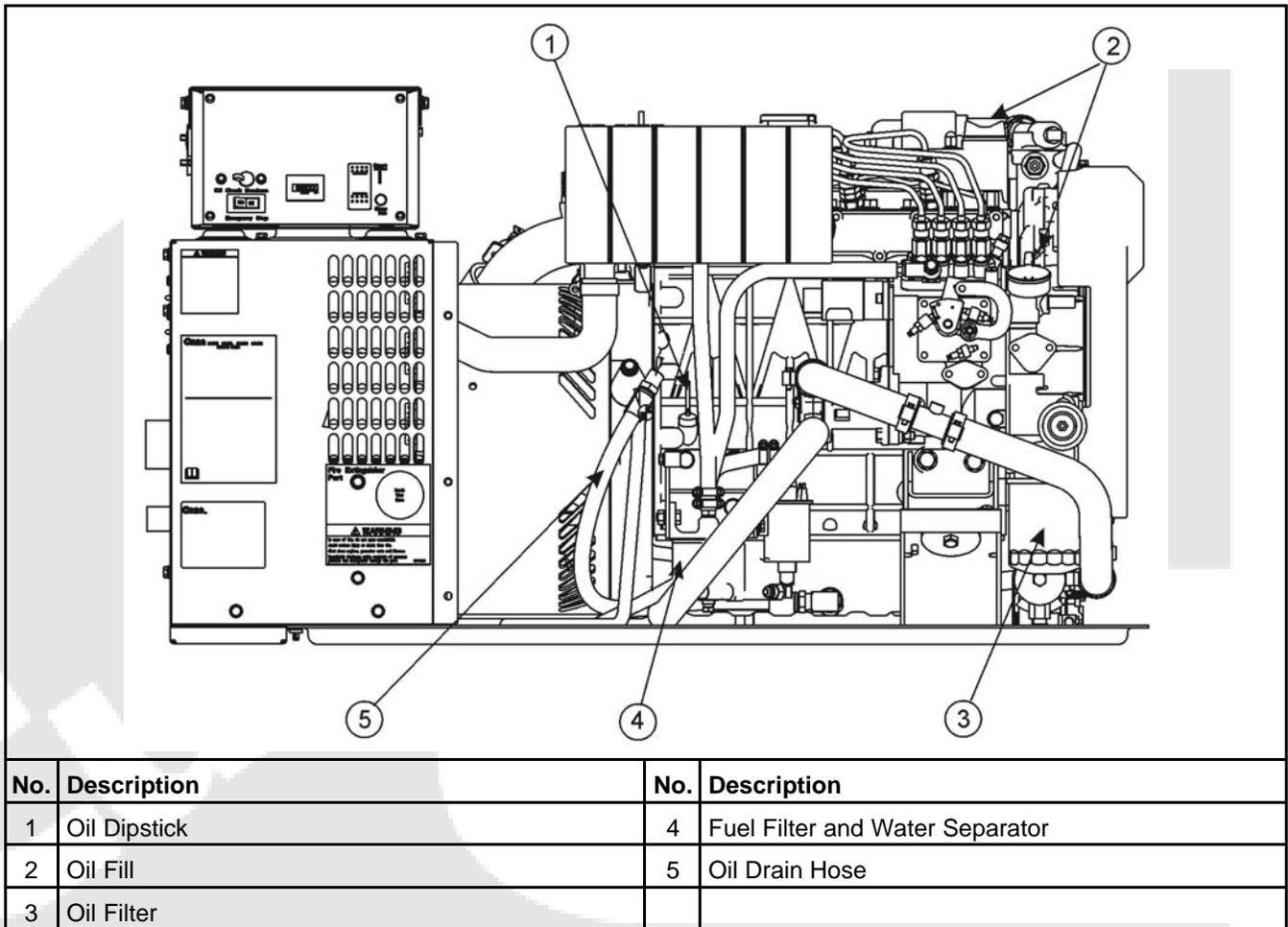
**FIGURE 13. OIL AND FUEL SERVICE POINTS - MDK BK, MDK BL, MDK BM, MDK BN**
