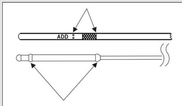
FIGURE 16. OIL LEVEL DIPSTICK ADD/FULL MARKINGS
