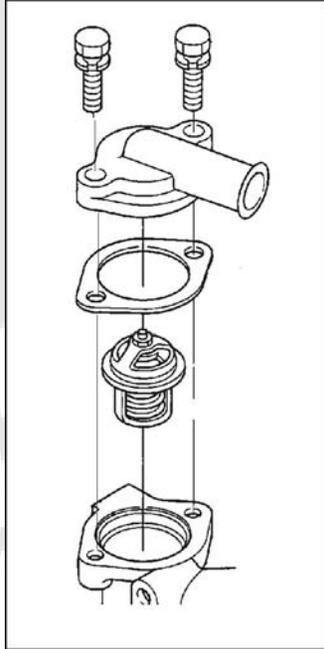
FIGURE 23. TYPICAL THERMOSTAT AND HOUSING
